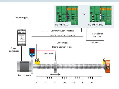
The ME versions of the modular small-scale controllers offer Ethernet, RS-485 or pulse/ direction interfaces. This means that electric motors can be driven by frequency inverters or other power electronics. In addition, limit switches and home position switches are connected directly to the controller.
