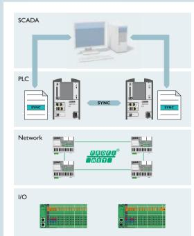
A redundant control system consists of various levels. The most important level is the control level, which has access to the process. Here, two compact controllers are synchronized in such a way that one of them always controls the process.
