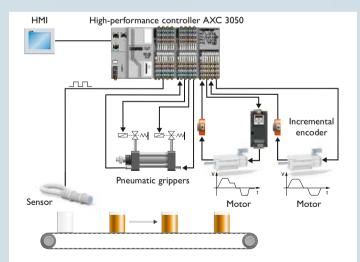
Medium-sized and large systems can be controlled in machine building using the modular AXC 3050 controller. Thanks to functions such as fast counters, high-performance processors, and direct I/O connection to Axioline F, you can perform demanding tasks, such as rotation speed and machine cycle monitoring.
