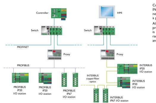
Conveniently connect your INTERBUS and PROFIBUS networks to the PROFINET using a proxy.
