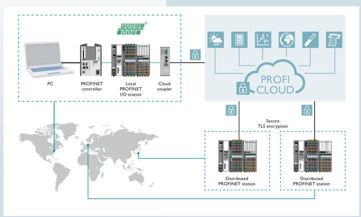
The cloud system for PROFINET for worldwide industrial communication consists of a Proficloud coupler, Proficloud controller,
